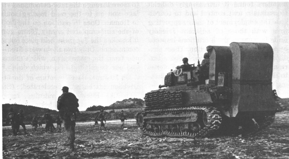
6TH DIVISION MARINES land on Oroku Peninsula. Note the medium tank with flotation gear. (USMC 122601)
