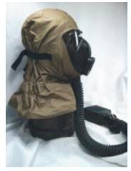
JSAM will be a lightweight CB protective mask that can be worn as CB protection for all aircrew. With the addition of anti-G features, it can be worn as combined CB and anti-G protection for aircrews in high performance aircraft. It will be compatible with existing CB ensembles, provide flame and thermal protection, provide hypoxia protection to 60,000 feet, and the CB portion will be capable of being donned in flight. JSAM will also be compatible with existing aircrew life support equipment.
