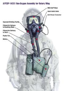
The CB Respiratory System is a self-contained protective ensemble designed for all forward deployed rotary wing (Version 1 for USN) and fixed wing (Version 2–4 for USN and USMC) aircrew. The design incorporates a CB filter, dual air/oxygen supply and a cross-over manifold with ground flight selector switch to provide filtered air for hood ventilation, and filtered air for oxygen for breathing. The system provides enhanced protection and offer anti-drown features.
