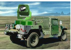
in a stand-off mode from a distance of 20 kilometers (km). The JSWILD/Artemis will operate from fixed sites ground vehicles, or shipboard. The system has distance-ranging and contamination-mapping capabilities and transmits this information to a battlefield information network.
