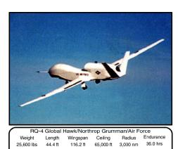
(Ku-band SATCOM) data links to its Mission Control Element (MCE), which distributes imagery to up to seven theater exploitation systems. ACTD residuals consist of four aircraft and two ground control stations. The Air Force has budgeted for two aircraft per year starting in FY02; IOC is expected to occur in FY05.
