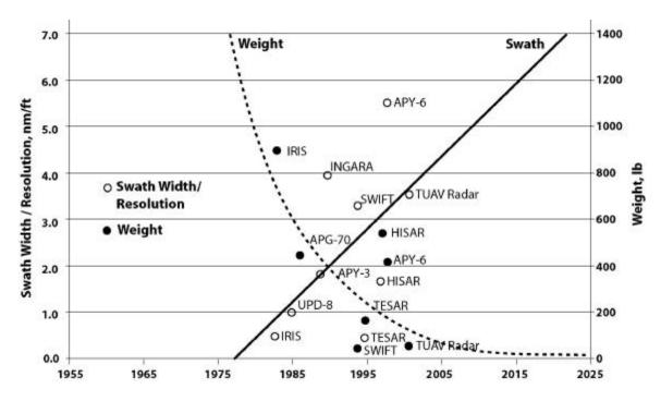
FIGURE 4.2.2-2: SAR WEIGHT AND COVERAGE/RESOLUTION TRENDS.
