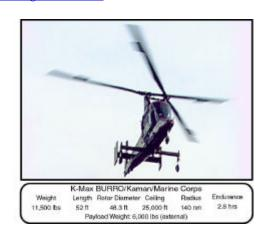
A converted K-Max helicopter is being used to explore the Marines' *Broad-area Unmanned Responsive Resupply Operations (BURRO)* concept of ship-to-shore or ship-to-ship resupply by UAV. It has been flying since early 2000.
