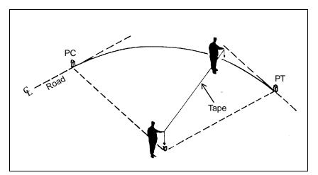
Figure I-3. Find the Radius with a Tape Measure
