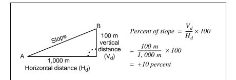
Figure I-5. Calculate the Percent of Slope
