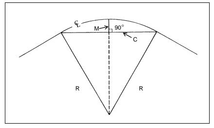
Figure I-4. Determine a Curve Radius
