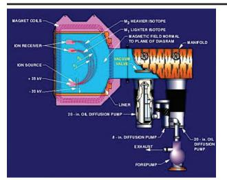
*Figure 18.* Example of EMIS separator and vacuum system.
