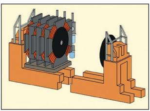
Figure 22. Schematic of the Iraqi EMIS machines.
