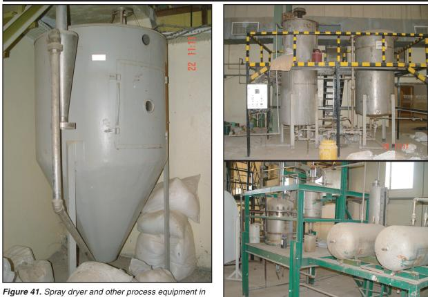
*Figure 41.* Spray dryer and other process equipment in Building 53.
