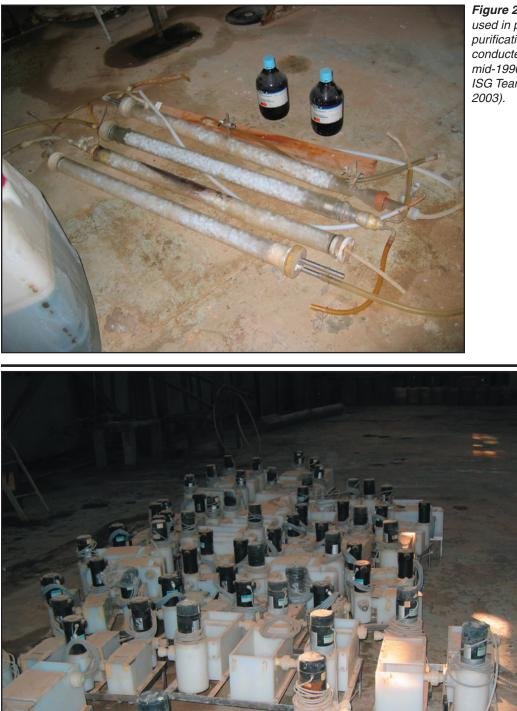
**Figure 25.** Packed columns used in phosphoric acid purification studies conducted at Ibn Sina in the mid-1990s (photo taken by ISG Team, December,
