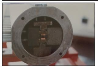
*Figure 29.* Cross-sectional view of Al-Tahadi rail gun showing how the rails are held with insulators and metal supports in a photo obtained from Hahdi Hadi Jasim.
