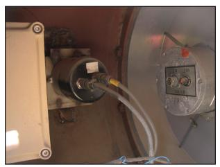
*Figure 16.* Submunition warhead safe, arm, fuze, and fire system located at the base of the warhead.
