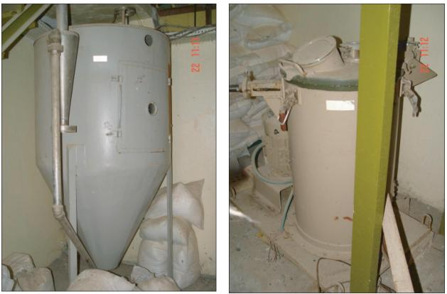
Building 53, Room 1. Dryer (left) and pressure vessel (right).
