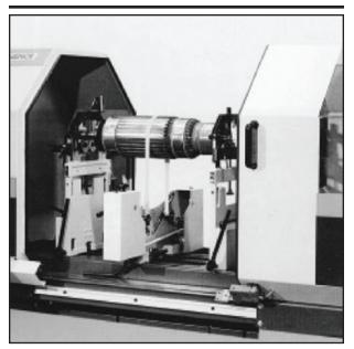
Figure 14. Typical horizontal balance machine.
