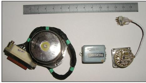
*Figure 28.* MG-4 gyroscope, AK-5 and A-15 accelerometers.
