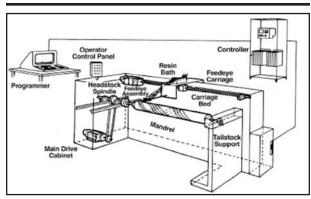
Figure 9. Horizontal filament winding machine.
