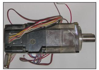
Figure 29. Actuator stepper motor.
