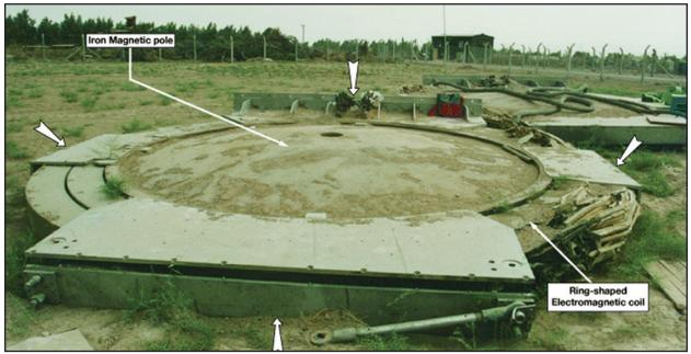
Figure 19. Photograph of Iraqi EMIS electromagnet.
