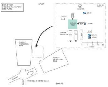
The secondary deployment area would represent the Command & Control (C&C) element of the PATRIOT system, consisting of the Information Coordination Central (ICC), the Tactical Command System (TCS), one of the Battery Command Posts (BCP), and their associated generators. The reason for the separation is the required distance between the antennas of the C&C element and the FCU. The secondary site would be on the Northwest side of the airport, near the intersection of Runways 14 and 20.
