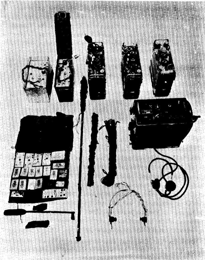
Communications Equipment Captured From an Enemy SIGINT Unit. (Top, left to right: a homemade transmitter, a homemade receiver, two U.S. AN/PRC-25's, and a U.S. AN/PRC-77. Bottom, left to right: radio receiver parts, antenna parts, wire, headphone, and a CHICOM R-139 receiver with headphone.)
