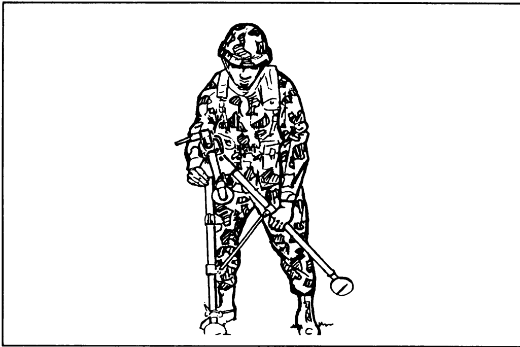
Figure 5-24. Folding the trail legs.
