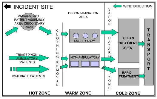
Figure 4-13. Emergency Decontamination Corridor System (2 Corridors)
