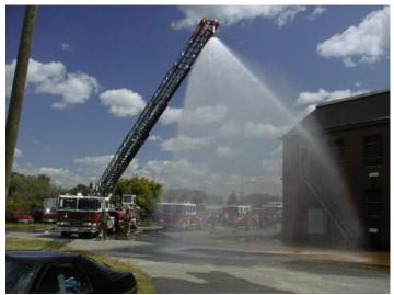
Figure 4-1. The Ladder Pipe Decontamination System
