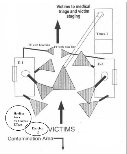
Figure 4-2. Schematic for Mass Decontamination
