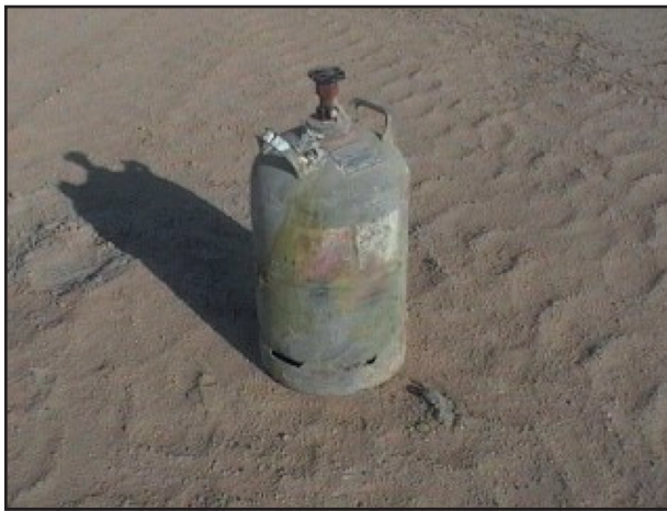
Figure 22. Tank of triethylamine recovered near Musayyib.
