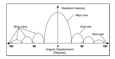
Figure 1: Example of an Antenna Pattern 23
